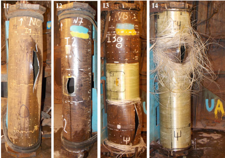
Fig. 7 Full-scale samples I1, I2, I3 and I4 after fracture by hydraulic inner pressure
