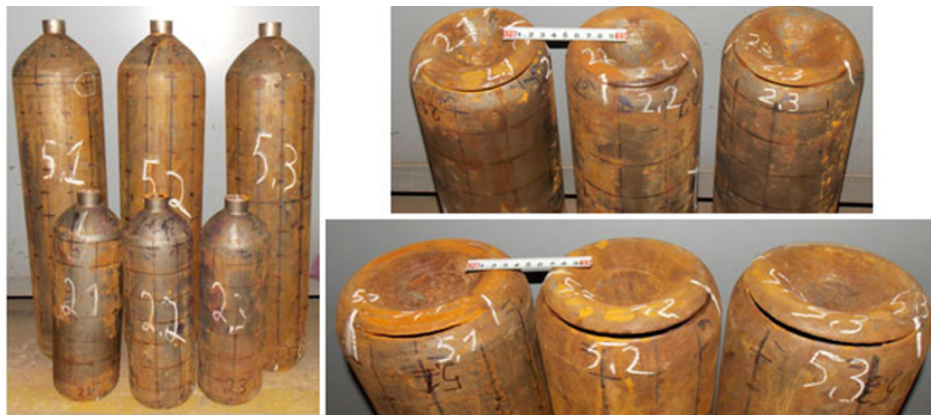
Fig. 3. Photographs of failed cylinders after cyclic hydraulic testing in their initial state and after failure.
