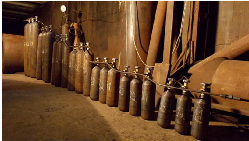
Fig. 1. Cylinders assembled in a garland for cyclic testing with test pressure.
