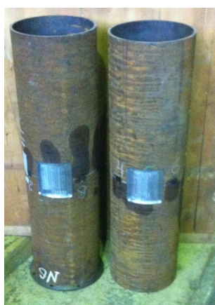
Fig. 14. Defects machined on two specimens
