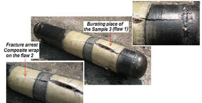
Fig. 6. Specimen 3 after testing (burst pressure: 31.5 MPa)
