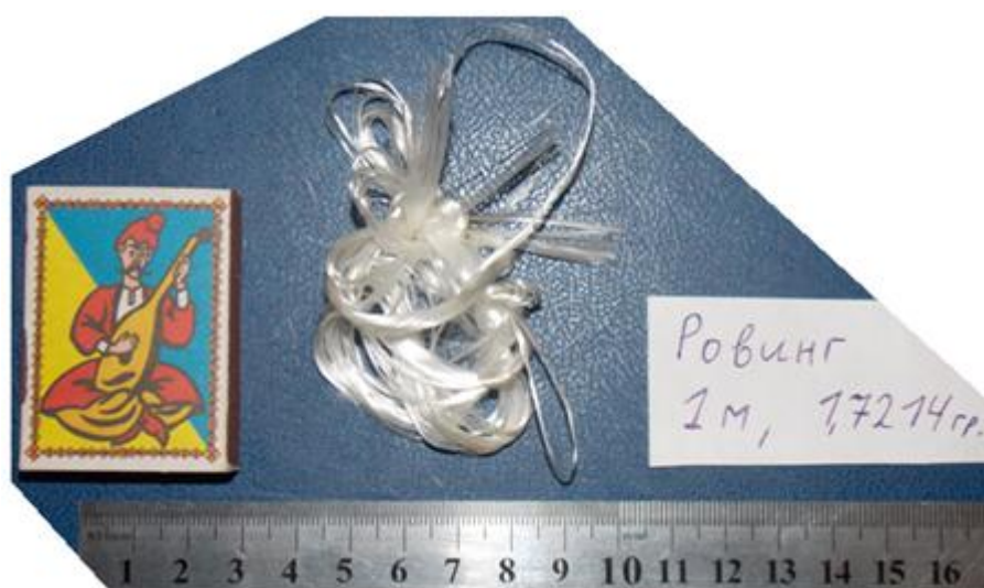
Figure 13. Specimen of the roving with length 1 m, subjected to weighing.
