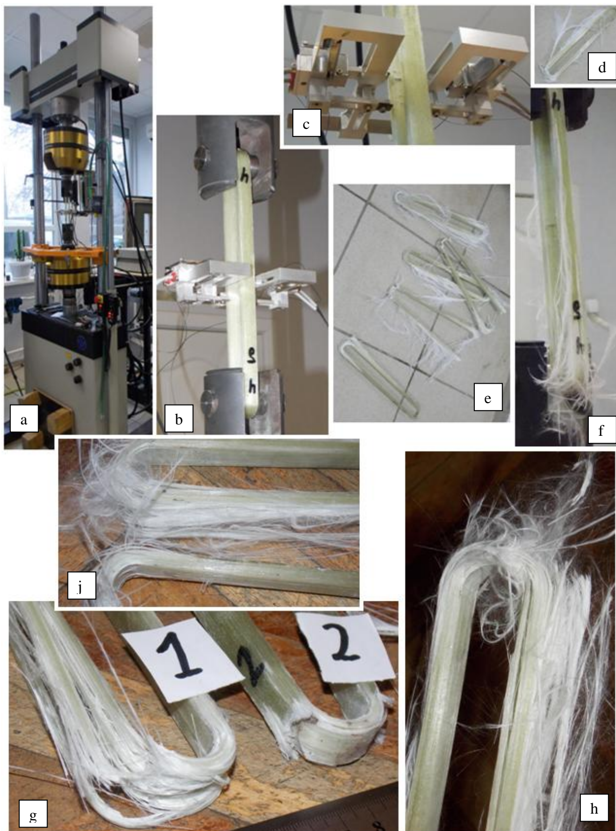
Figure. 4. Tensile test: a - testing machine Instron 8802; b - specimen gripping; c - extensometer Biaxial 2620-614; d, e, f, j, g, h - features of specimens fracture.
