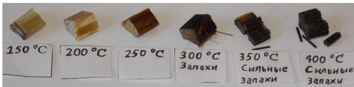
Figure. 15. Elements of the specimens after half an hour exposure excerpts to different temperatures.
