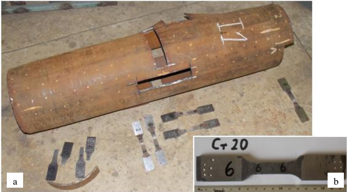
Fig.10. Sample for tensile test cut out the specimen II after its destruction.
