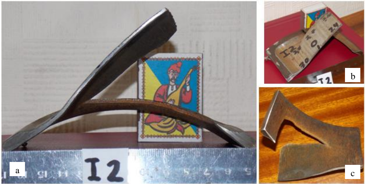
Fig. 19. Fracture in defect zone.
