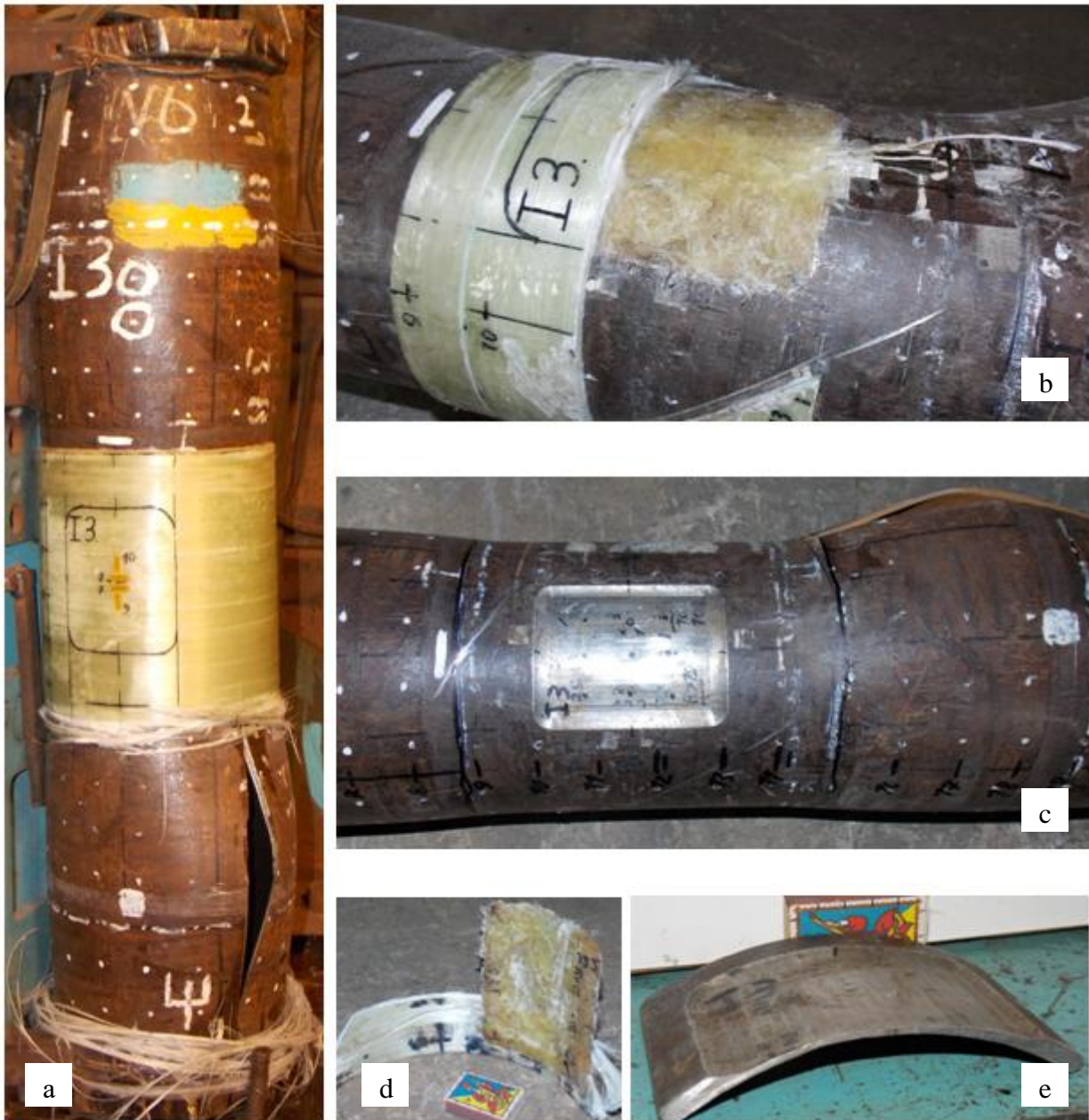
Fig. 29. Specimen I3 after the destruction: a sample after the test; b - in the process of disclosure of the defect; c - after the complete opening of the defect; d - filling of the defect; e – the cut area of the defect.
