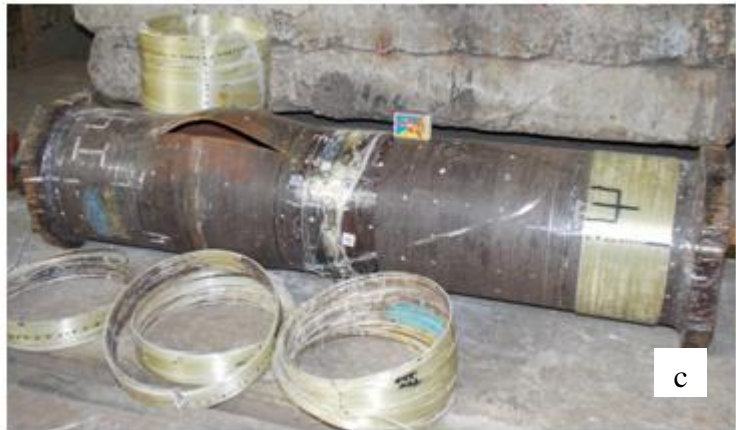
Fig. 36. Specimen (a) - after the destruction; (b, c) - after removal of the bandage.
