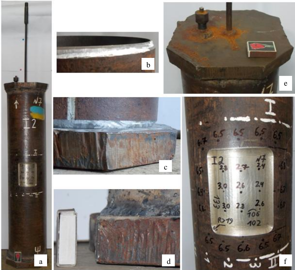
Fig.12. Specimen I2: a - before the test, b – pipe edge prepared for welding; c, d - welding of the lower bottom; e - top end of the specimen; f - defect (numbers near the points indicate the wall thickness).
