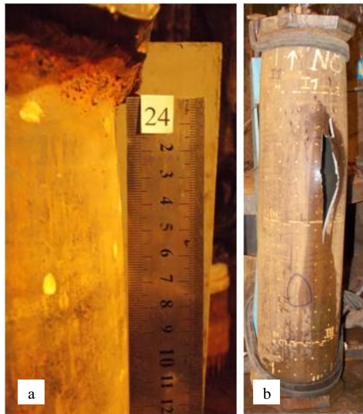
Fig. 9. Specimen II. a - after step 24; b - after failure (step 25).
