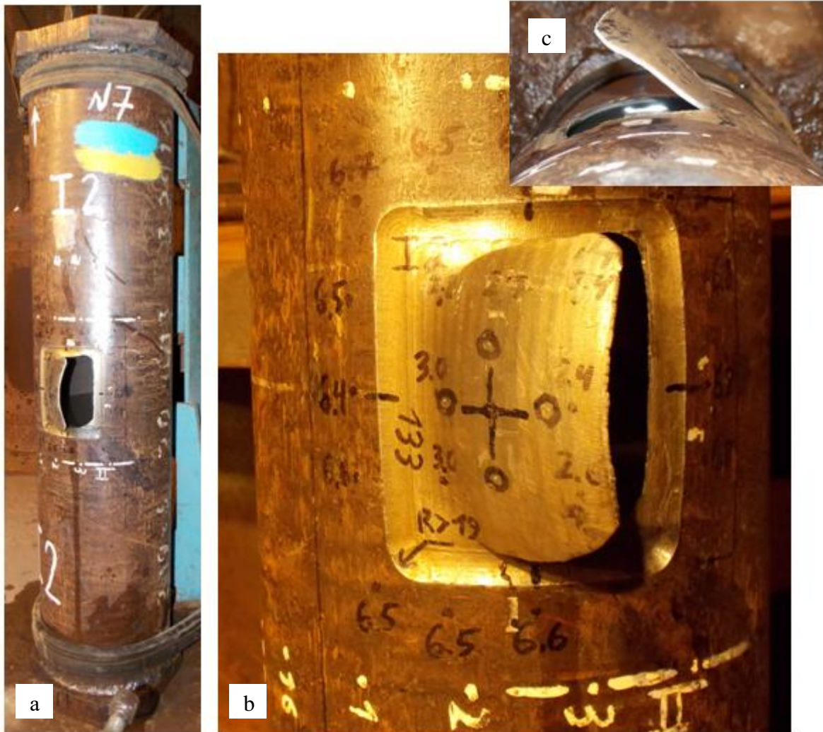
Fig.17. Destruction of the specimen: a - general view; b, c - the destruction in the defect.
