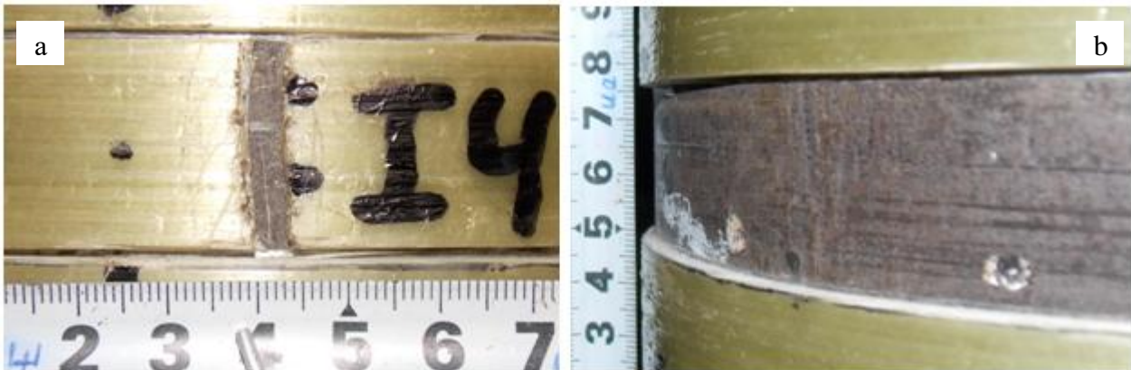
Fig. 32. Axial groove in the ring (a); bandage after removal of the ring (b).
