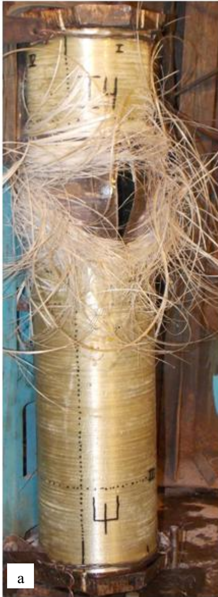
Fig. 36. Specimen (a) - after the destruction; (b, c) - after removal of the bandage.
