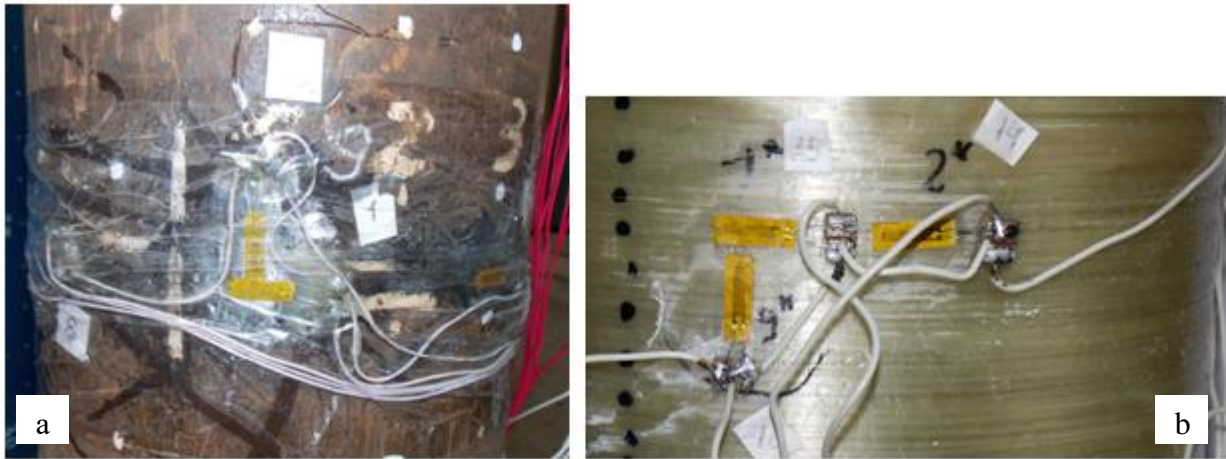
Fig. 33. Strain gages on the surface of the pipe before installing the bandage (a) and at the bandage surface (b).
