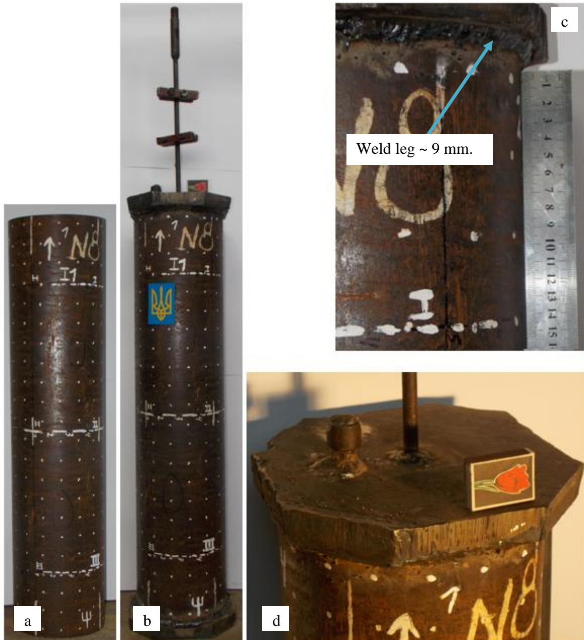
Fig. 3. Specimen I1 (points indicate places of the measurement thickness): a – pipe piece #8; b - specimen before the test; c - welding of the pipe; d - top bottom with the fittings.
